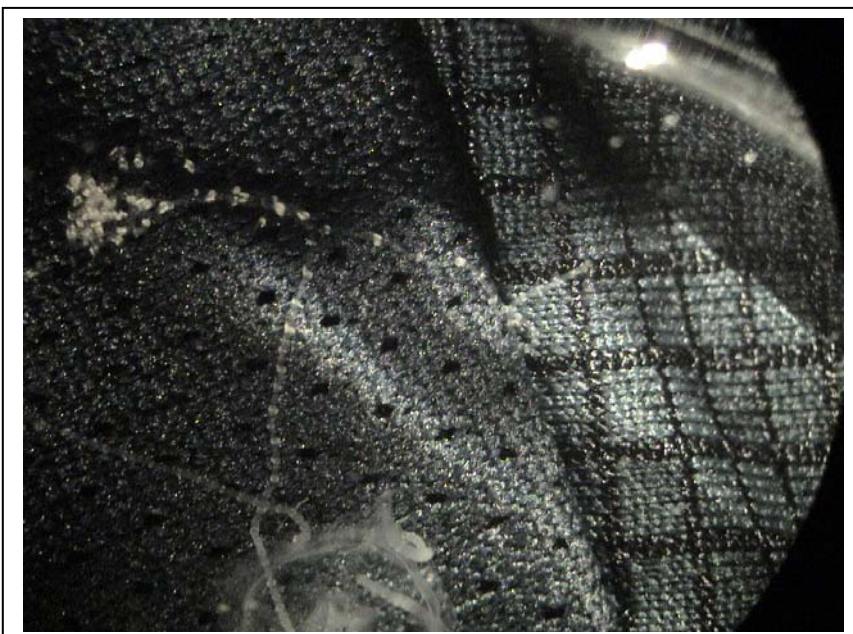
Figure 11. Carukia barnesi tentacles and the Nike Dri-Fit sport shirt. Note two types of weave in the test area, a weave with regularly-spaced small holes to the left, and a closed weave to the right.
